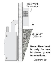
\*Dia 3, 3a & 4: As specified in CGA B149 Installation Code. Local codes or regulations may require different clearances.
